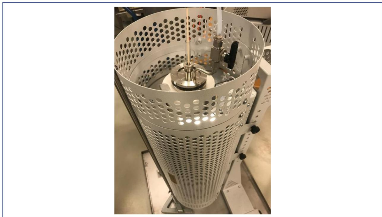
Figure 8.1: Photo of test furnace with melting cell. In the middle is a quartz tube with a thermal sensor and a connection to argon shielding gas. The melting cell itself with the phase-shifting material (AlSi12) is not visible, but is shown in Figure 8.3.
