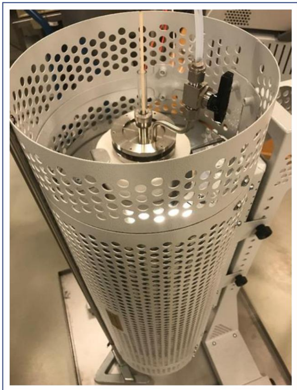
Figure 4.2: Photo of test furnace with melting cell. In the middle is a quartz tube with a thermal sensor and a connection to argon shielding gas. The melting cell itself with the phase-shifting material (AlSi12) is not visible.
